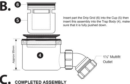
Can be installed with or without optional 45 degree bend.
