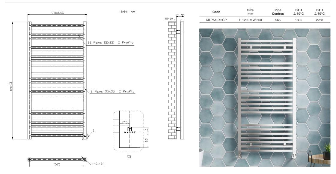
Please note due to manufacturing tolerances pipe centres may vary by +/- 10mm, we recommend that pipe work is not altered until your towel rail / radiator is on site. The information contained on this page was correct at date of issue. Fitting dimensions are provided as a guide only. We pursue a policy of continuing improvement in design and performance of our products and so reserve the right to change specifications without prior notice.
