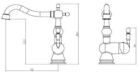
Construction Brass Body CuZn40Pb2, EN CW617N (equivalent to BS CZ122)
