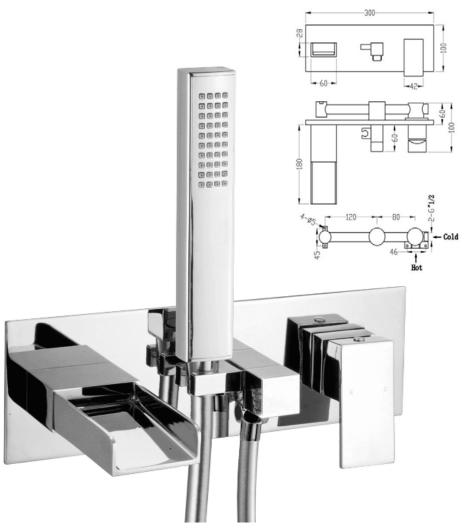
Construction Brass Body CuZn40Pb2, EN CW617N (equivalent to BS CZ122)
