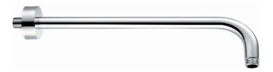
Construction Finishes Product Type Plumbing Systems Fitting Guarantee Brass Body (CuZn40Pb18) Chrome plated to BS EN 248 Contemporary Suitable for all plumbing systems G1/2" BSP 10 years against manufacturing faults (3 Years on Serviceable Parts).
