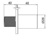
Construction Finishes Product Type Plumbing Systems Fitting Guarantee Brass Body (CuZn40Pb18) Chrome plated to BS EN 248 Contemporary Suitable for all plumbing systems G1/2" BSP 10 years against manufacturing faults (3 Years on Serviceable Parts).
