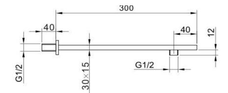
Construction Finishes Product Type Plumbing Systems Fitting Guarantee Brass Body (CuZn38Pb18) Chrome plated to BS EN 248 Contemporary Suitable for all plumbing systems G1/2" BSP 10 years against manufacturing faults (3 Years on Serviceable Parts).
