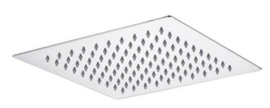
Construction Stainless steel 304 **Finishes** Chrome **Product Type** Contemporary Water Pressure Min 1.0 bar and Max 5.0 bar **Plumbing Systems** Suitable for all plumbing systems Weight(net) 0.75kg/piece Fitting G1/2" Guarantee 10 years against manufacturing faults (3 Years on Serviceable Parts).
