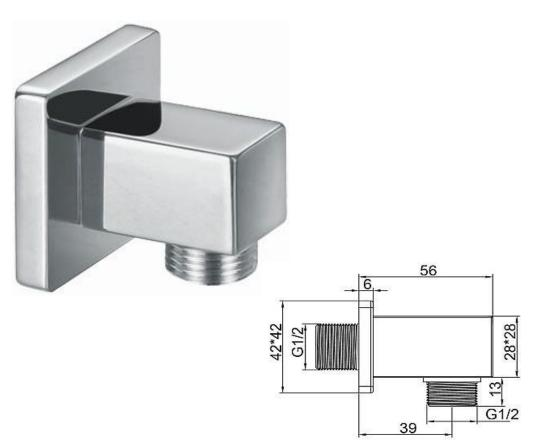
Construction Finishes Product Type Plumbing Systems Fitting Guarantee Brass Body (CuZn40Pb18) Chrome plated to BS EN 248 Contemporary Suitable for all plumbing systems G1/2" BSP 10 years against manufacturing faults (3 Years on Serviceable Parts).
