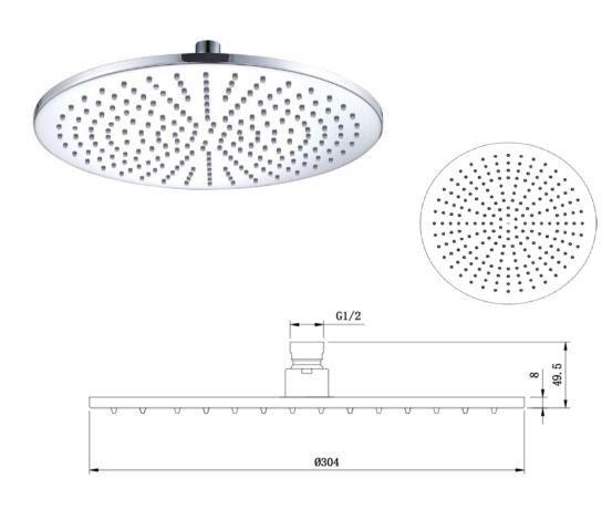
ConstructionBrass Body (CuZn38Pb18)FinishesChrome plated to BS EN 248
