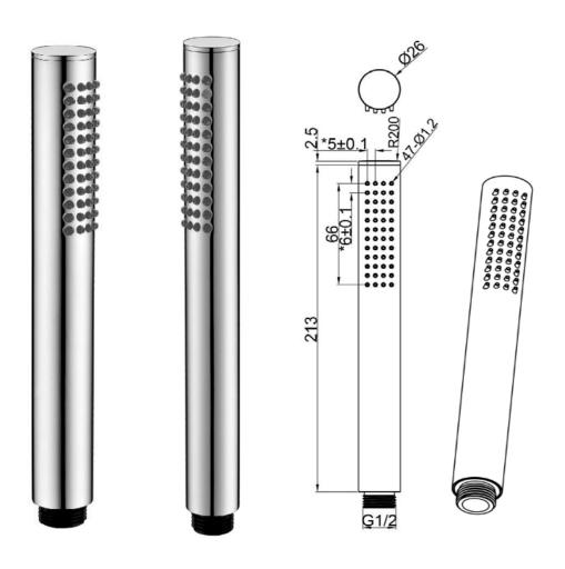
Brass Body CuZn40Pb2, EN CW617N (equivalent to BS CZ122) Construction
